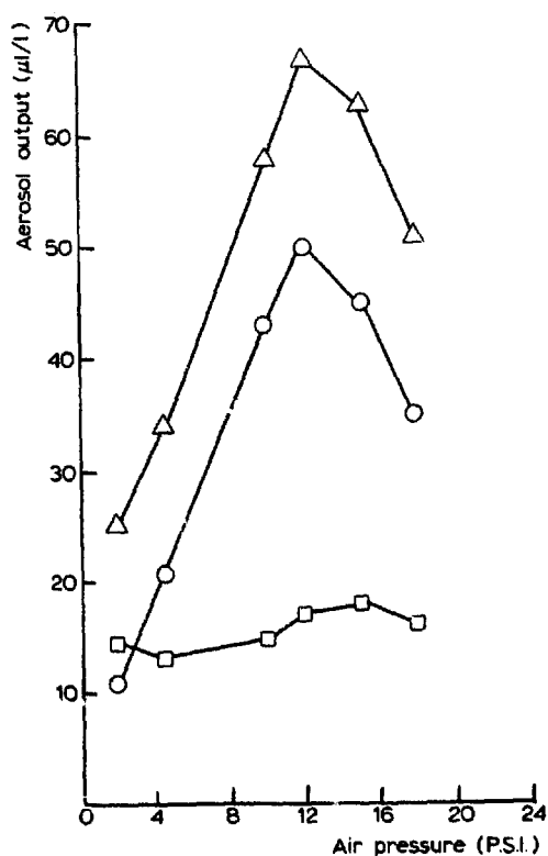
Fig. 7. The effect of air pressure on aerosol output (50% w/v propylene glycol solution). Δ, total output; ○, solution output; □, vapour output.
